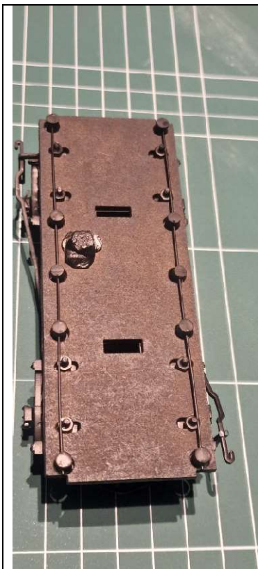
Fig 1 and 2 shows the wire holding the brake gear in place
