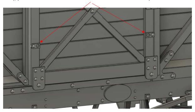
You may have to drill them out slightly to get the brass to fit nicely for gluing.
