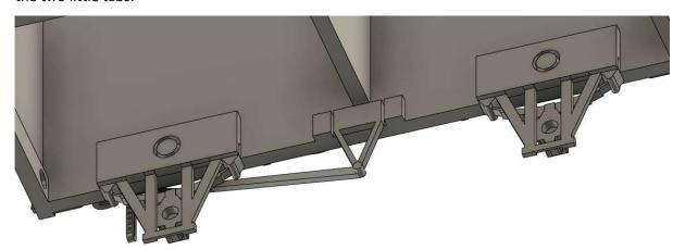
To do the other side, I would recommend loosely mounting the wheels in without glue for now, in order to check the tolerance of the brake blocks.
