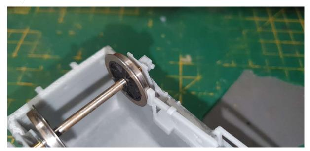
You can now check the brake blocks against the wheels and the brake lever on that side:
