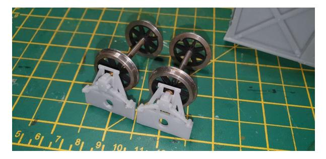
You will then place the open end in the axle box already mounted, and the still loose axle box should fit right in:
