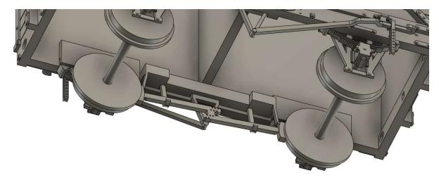
I would then recommend leaving the final gluing of the wheels and second pair of axle boxes until the model as been painted, in order to make it easier to not paint the wheels.
