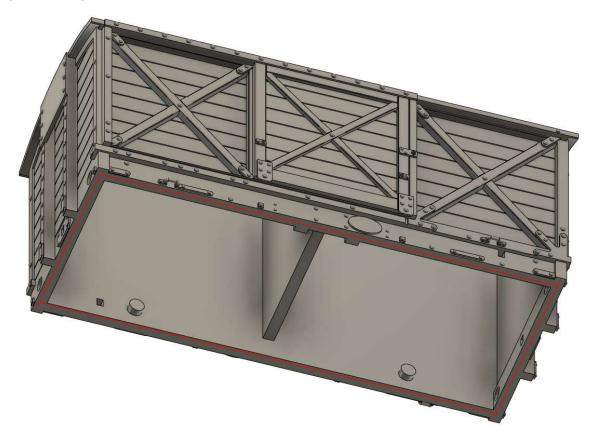
The next thing you will need to do it test fit the brake lever into these holes on the side, they may need to be filed out a tad in order to fit better: \
