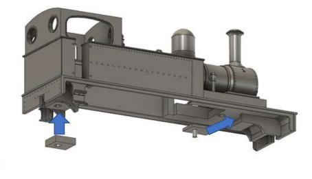
Spacers for use with Graham farish chassis. Front spacer fits to chassis with peg locating in hole between cylinders. the chassis then slides into postition with the spacer going into the slot in the chassis.
