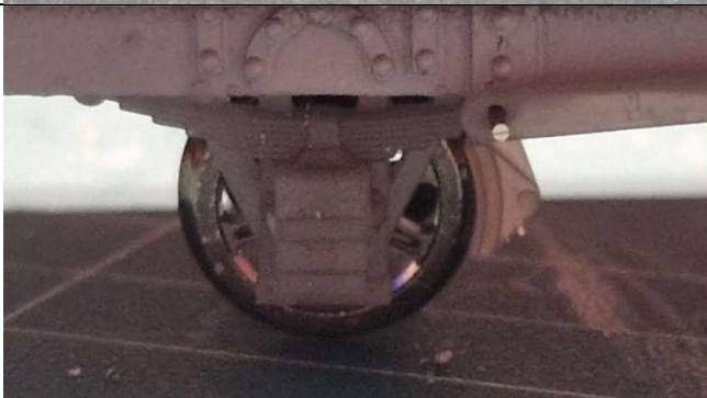
Glue a piece of brass into the brake block and slide it into place on the axle unit.
