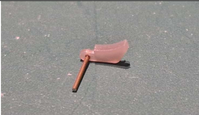
Glue a piece of brass rod into the brake arm pivot point
